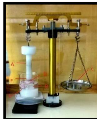
Fig. 1: Modified mucoadhesion test apparatus (Fabricated)
