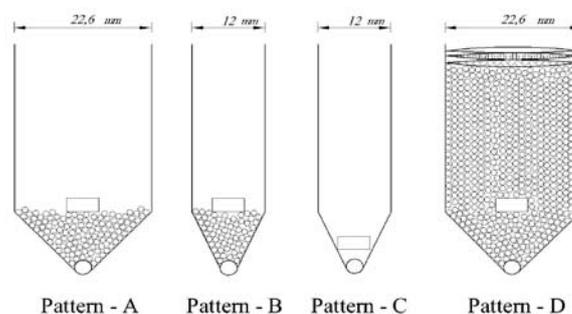
Fig. 1: Schematic diagrams showing the four patterns for MX tablet loaded into the FTC
