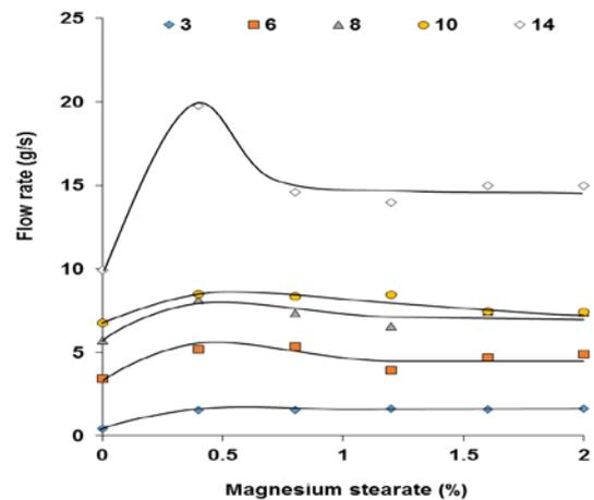
**Fig. 6: Effect magnesium stearate on the flow rate of GalenIQ 720, assessed with glass funnels with openings of different size (mm).**
