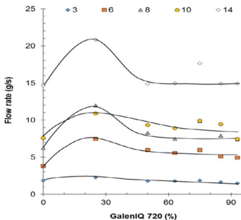
**Fig. 9: Effect of GalenIQ 720 on the flow rate of its mixtures with metronidazole, assessed with funnels with different size openings (mm).**
