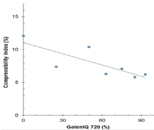
**Fig. 8: Effect of different proportions of GalenIQ on the compressibility index (%) of metronidazole.**
