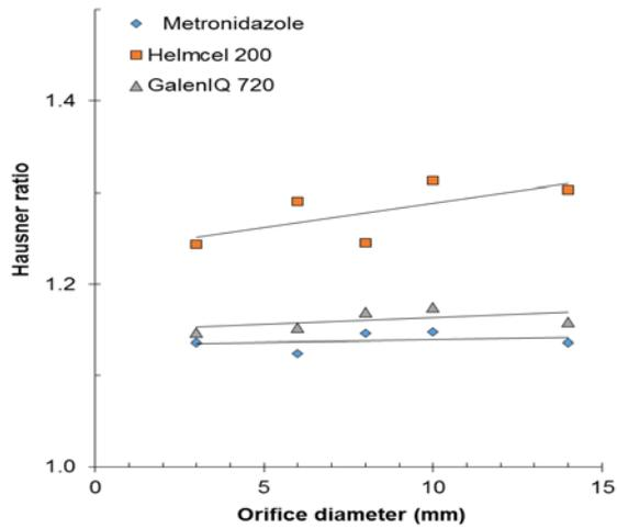
**Fig. 2: Hausner ratio values obtained for GalenIQ 720, Helmcel 200 and Metronidazole, using funnels with orifices of different size.**
