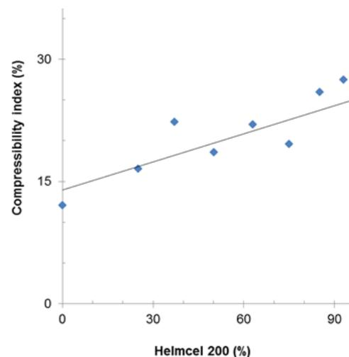
**Fig. 11: Effect of the Helmcel 200 proportion on the compressibility index of its mixtures with metronidazole, expressed as the average obtained when using funnels with different size openings.**
