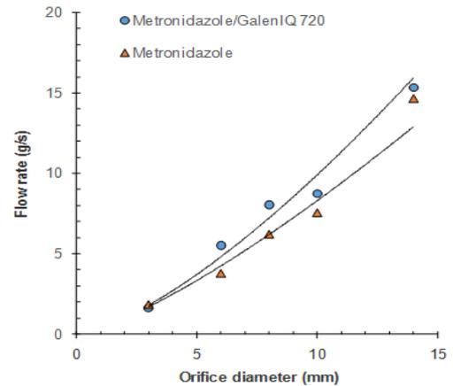
**Fig. 10: Effect of the orifice diameter on the flow rate of metronidazole and its mixtures with GalenIQ 720.**
