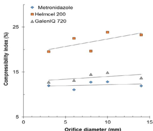
**Fig. 1: Compressibility indexes (%) obtained for GalenIQ 720, Helmccl 200 and Metronidazole, using funnels with different opening sizes.**
