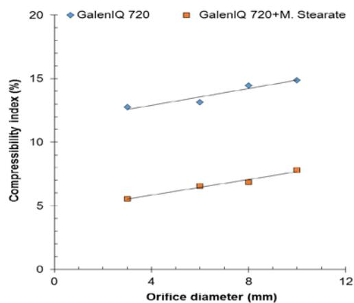
**Fig. 5: Effect of the orifice diameter and the addition of magnesium stearate on the compressibility index of GalenIQ 720.**
