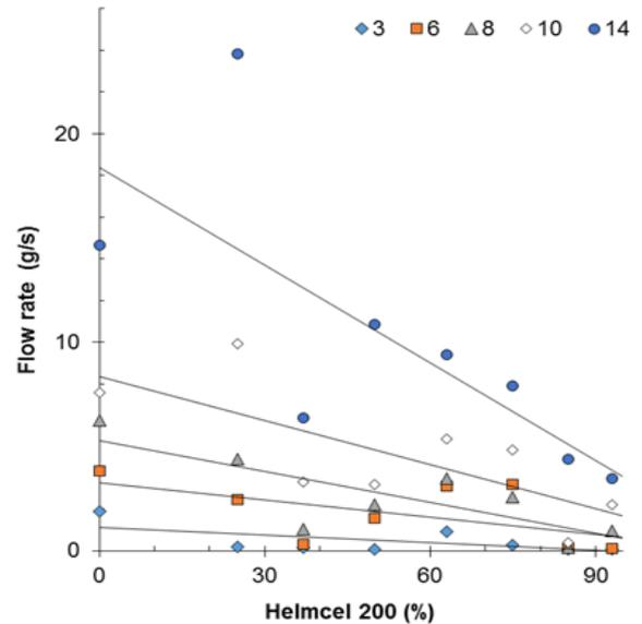
Fig. 12: Effect of the Helmcel 200 proportion on the powder flow rate of its mixtures with metronidazole, measured with funnels with different size openings (mm).
