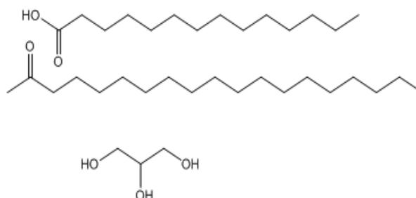
Fig. 2: Structure of Precirol ATO 5
