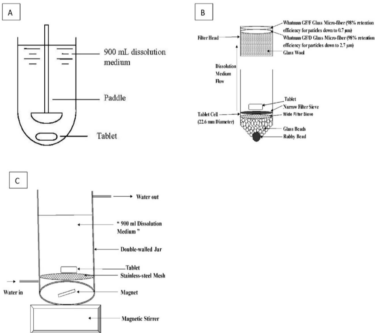
Fig. 1: Schematic diagrams of: (A) USP apparatus II, (B) USP apparatus IV, (C) Beaker method
