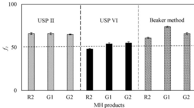
Fig. 3: Comparison between dissolution profiles of different MH IR market products (R2, G1, G2) versus R1 (Glucophage®) expressed by the similarity factor " $f_2$ ", utilizing different apparatuses (mean±SD, n = 3)
