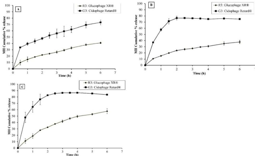
Fig. 4: Dissolution profiles of two MH CR products obtained using: (A) USP apparatus II, (B) USP apparatus IV, and (C) Beaker method (mean $\pm$ SD, n=3)
