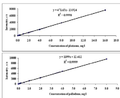
**Fig. 2: Calibration curve for concentration of platinum (Pt) and palladium (Pd) ( $\mu\text{g/l}$ ) vs emission intensity (c/s) by ICP-OES**
