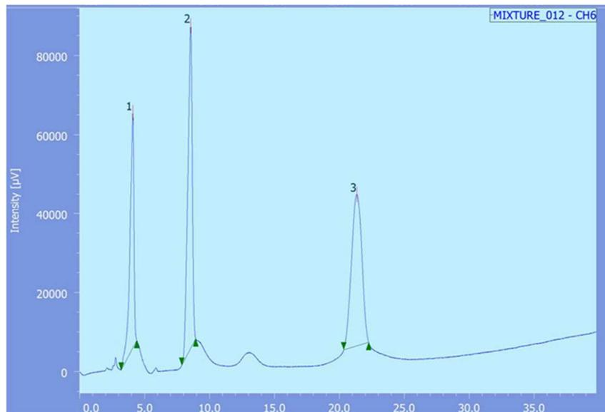
Fig. 6: HPLC chromatogram of a 20 µl injection of a standard mixture of 0.1 µg/ml TRT, 8 µg/ml HQ and 1 µg. ml<sup>-1</sup> HC using the optimized chromatographic conditions
