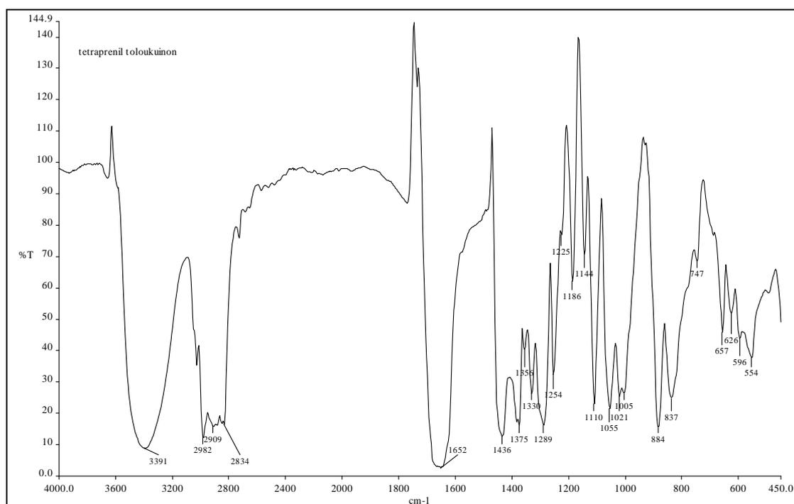
Fig. 1: FTIR spectrum of TPTQ in nujol
