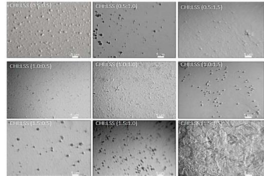
**Fig. 2: Optical micropictures of AA microcapsules obtained by ultrasonication-homogenization**
