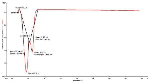
Fig. 5: DSC of stearic acid, pluronic F 68 and tripalmitin
