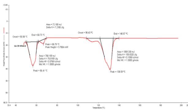
Fig. 6: DSC for stearic acid, tripalmitin, pluronic-F-68 and etoricoxib
