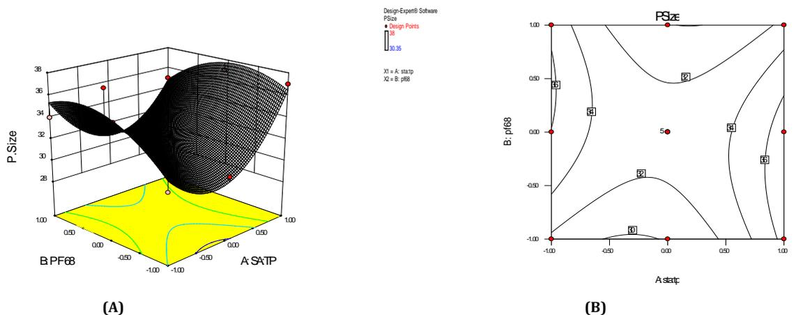
**Fig. 2: (A) Response surface plot showing the influence of stearic acid: tripalmitin and the amount of pluronic F-68 on particle size and (B) corresponding contour plot showing the relationship between various levels of lipid ratio and amount of surfactant**
