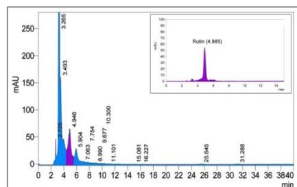
**Fig. 7: HPLC chromatogram of MEMT at 254 nm insert within image reference standard Rutin**
