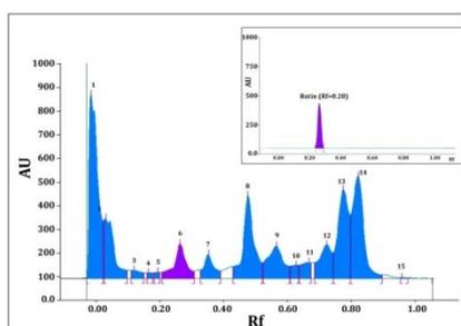
**Fig. 4: HPTLC Chromatogram of MEMT and the insert with in the image shows the reference standard Rutin**
