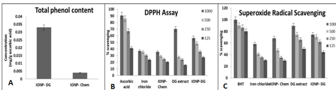
**Fig. 6: Free radical scavenging activity and total phenol content of IONPs**
