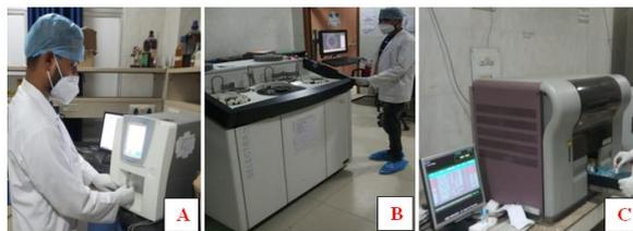
Fig. 1: (A) Medonic three hematology analyzer; (B) Selectra machine for biochemical analysis; (C) Stago machine for coagulation tests
