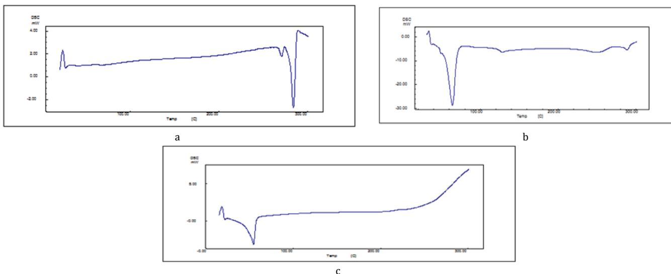
Fig. 18: DSC thermograms of (a) TA, (b) physical mixture of TA - GMS and (c) TA- SLNs (formula F1)
