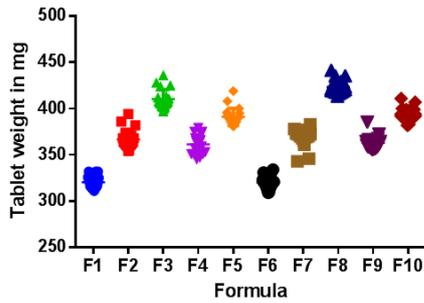
Fig. 2: Weight variation %RSD of different matrix formulations (N is 20 tablets per formulation run)
