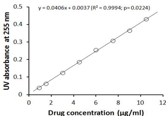
Fig. 1: UV calibration curve of standard Ketoprofen in pH 6.8 phosphate buffer measured at  $\lambda_{\max}$  255 nm. Each data point is the average of three determinations
