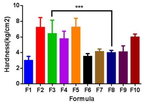
Fig. 4: Hardness of different matrix formulations (N is 10 tablets for each formulation run. Data are shown as mean ± SD)
