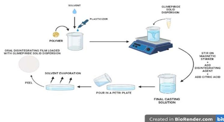
**Fig. 1: Schematic representation of preparation of fast-dissolving buccal film loaded with Glimepiride solid dispersion**
