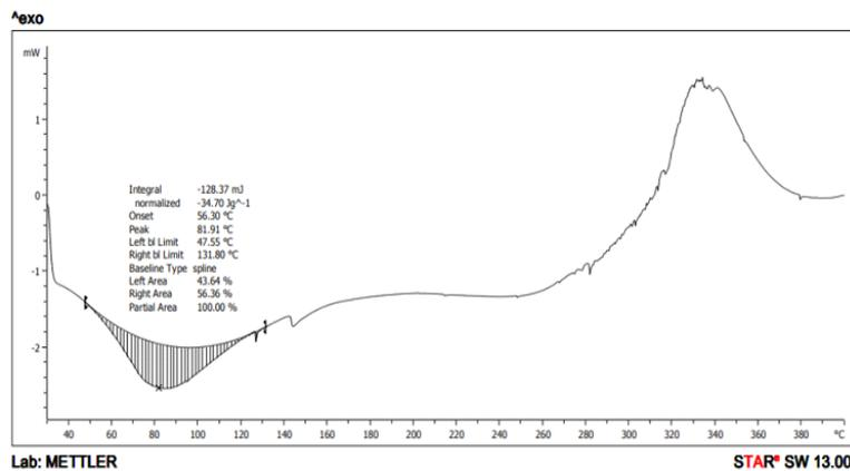
Fig. 11: DSC thermogram of optimised solid dispersion
