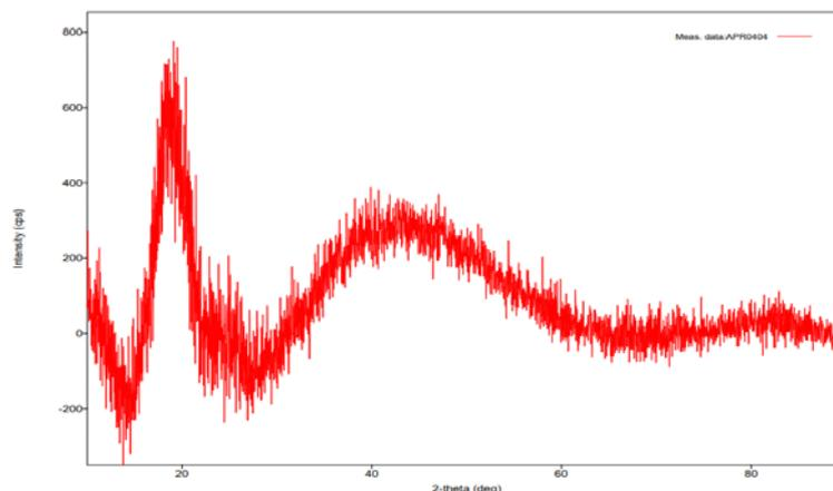
Fig. 28: XRD pattern of optimised film
