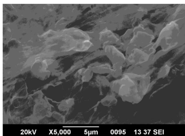
Fig. 29: SEM image of the optimised film (X5000)
