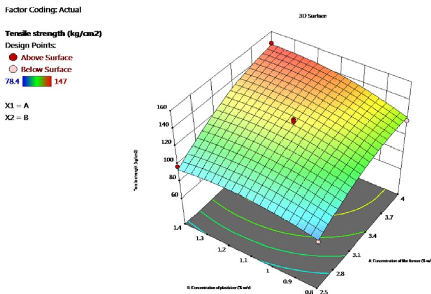
Fig. 24: 3D surface plot of effect of A and B on tensile strength
