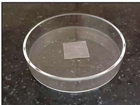
Fig. 25: Optimised glimepiride solid dispersion loaded FDBF
