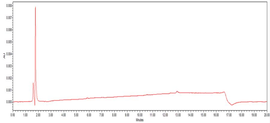
**Fig. 3: Typical chromatogram of placebo solution**
