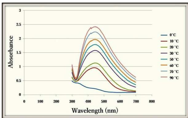
Fig. 2: UV spectral peak of temperature dependent silver Nanoparticles synthesized at different temperature
