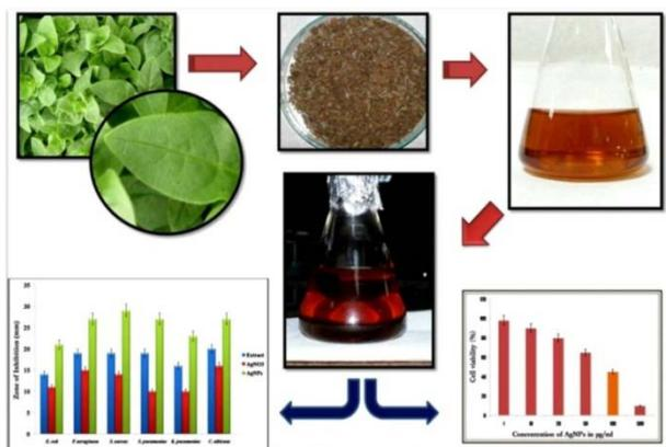
**Fig. 12: Schematic diagram of synthesis of AgNPs from *O. heracleoticum* L**
