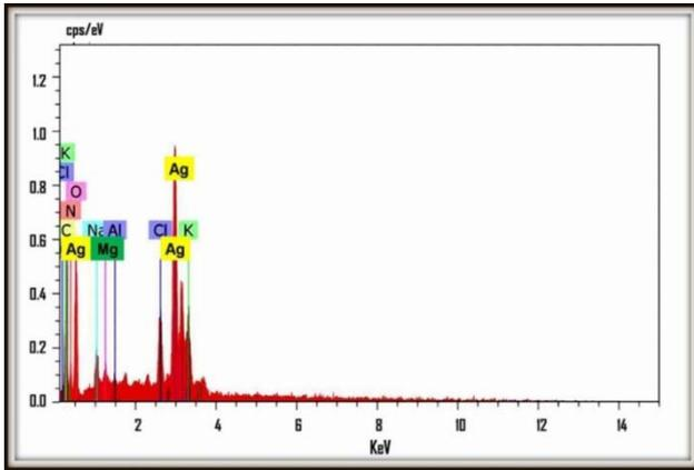
Fig. 7: Energy dispersive X-ray spectrum of Nanoparticles
