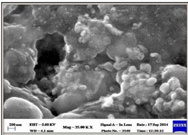
Fig. 3: Field emission-scanning electron microscopic image of AgNPs
