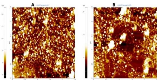
Fig. 6: AFM micrographs of PLAN and Q-PLAN (F3)
