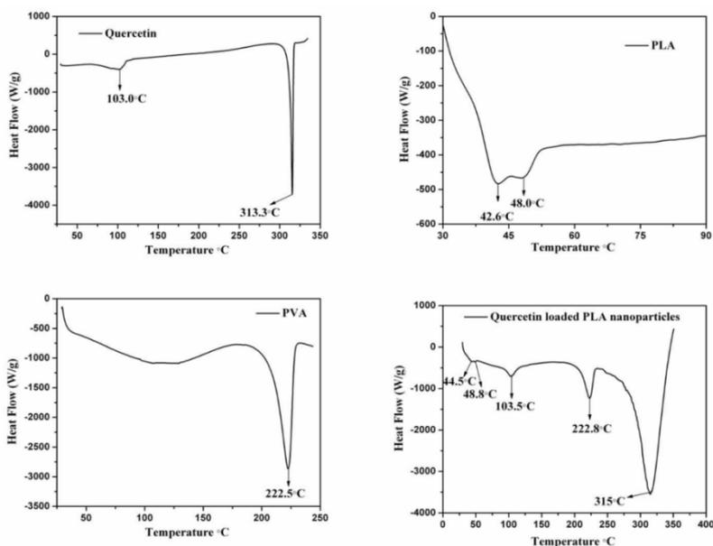
Fig. 1: DSC thermograms of free quercetin, PLA, PVA and Q-PLAN
