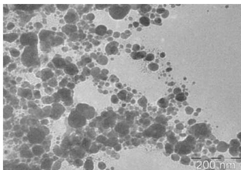
Fig. 4: TEM image of formed silver nanoparticles
