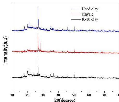
**Fig. 1: XRD patterns of Clay, Clayzic and used clay catalysts**
