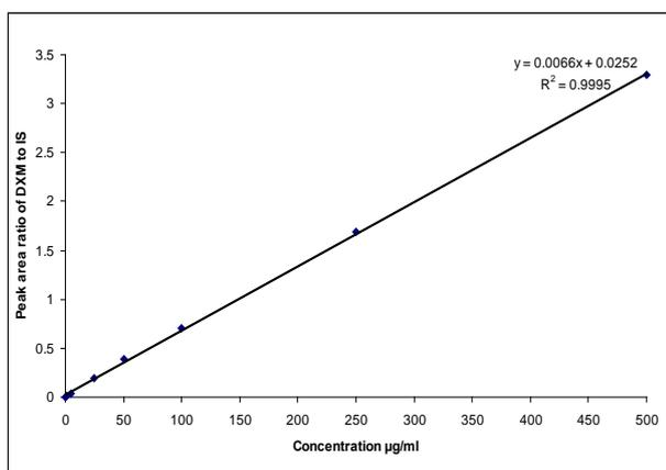
Fig. 4: Linearly regressed calibration curve of dexamethasone
