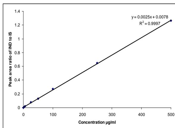
Fig. 5: Linearly regressed calibration curve of indomethacin
