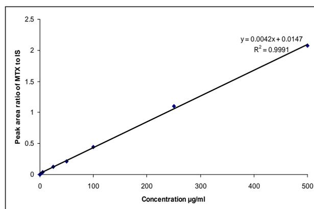
Fig. 3: Linearly regressed calibration curve of methotrexate
