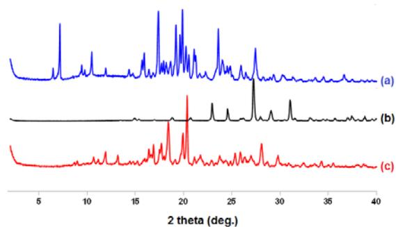
Fig. 3: PXRD pattern of KTZ (a), OXA (b), KTZ OXA (c)
