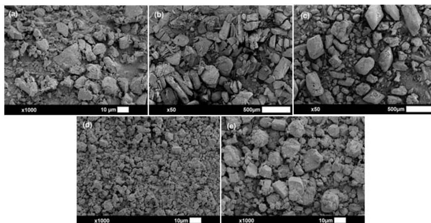
**Fig. 6: SEM images of KTZ (a), FUMA (b), OXA (c), KTZ FUMA (d), KTZ OXA (e)**
