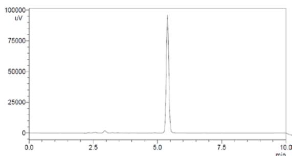
**Fig. 9: Cephalexin in urine sample injected as it is after 8 hours of oral administration**
