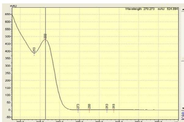
Fig. 2: The optimum wavelength for detection was used at 232 nm
