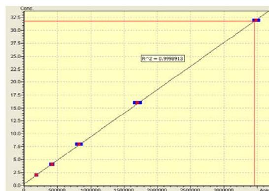
Fig. 3: HPLC Linearity graph for metformin ( $r^2=0.99980$ )
