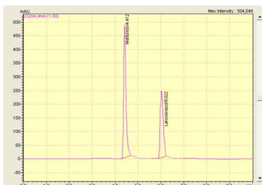
**Fig. 4: HPLC-UV chromatogram obtained human plasma sample after metformin administration (retention time 4.41 min), and HPLC-UV chromatogram obtained for internal standard (6.022 min)**
