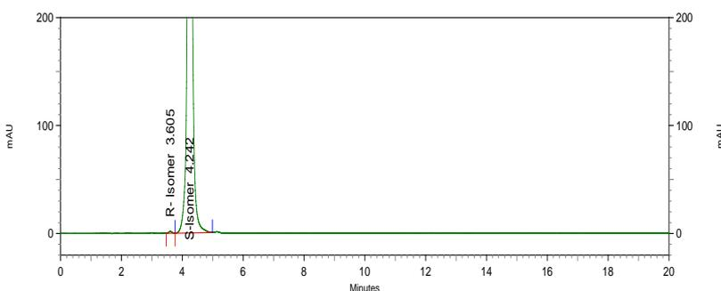
Fig. 5: Typical HPLC chromatogram of Etodolac bulk sample (100 µg/ml) spiked with R-isomer (0.2 %)
