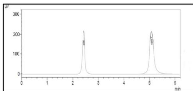
Fig. 5: Chromatogram of standard (Urine Matrix+ISTD+Drug)
