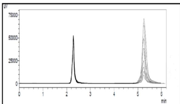
Fig. 6: Overlay chromatogram of standard solution
