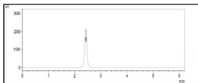
Fig. 4: Chromatogram of double blank (Urine Matrix+ISTD)
