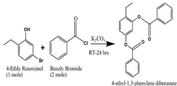
Fig. 4: Scheme for the synthesis of CqsER-4
