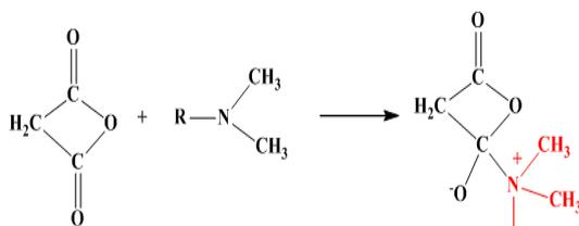
**Scheme 1: Proposed reaction pathway between MAA and APT under the described reaction conditions**
