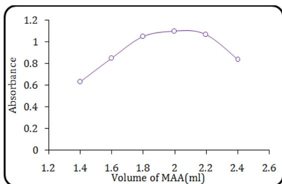
**Fig. 4: Effect of volume of MAA (8%w/v) on the absorbance value of the reaction product of APT (10µg/ml) with MAA**
