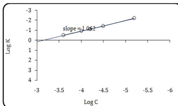
**Fig. 8: Linear plot for  $\log C$  versus  $\log K$  for the kinetic reaction of APT with MAA. C is the APT concentration ( $1.3 \times 10^{-4} - 1.9 \times 10^{-4} \text{ M}$ ) and  $K$  is the reaction rate ( $\text{second}^{-1}$ )**
