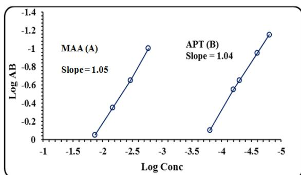
**Fig. 7: Limiting logarithmic plot for molar reactivity of APT with MAA. C and A are the concentration and absorbance, respectively. For generating the first line (A), MAA:  $[1.7 \times 10^{-3} - 13.6 \times 10^{-3} \text{ M}]$ ; APT:  $[1 \times 10^{-4} \text{ M}]$ . For generating the second line (B), APT  $[7.5 \times 10^{-6} - 2.5 \times 10^{-4} \text{ M}]$ ; MAA:  $[1.7 \times 10^{-3} \text{ M}]$**
