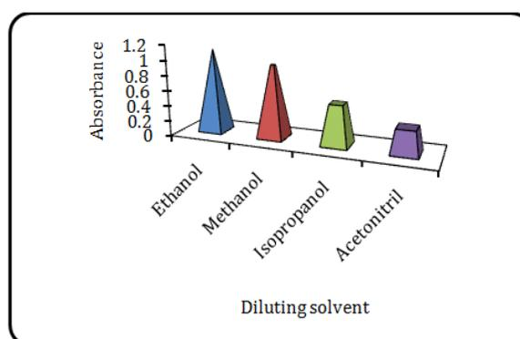
**Fig. 5: Effect of diluting solvent on the absorbance of the reaction product between APT (10µg/ml) with MAA (8%w/v)**
