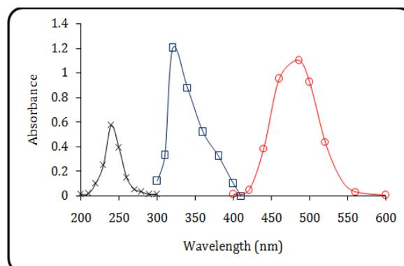
Fig. 2: Absorption spectra of: (a) APT (10µg/ml) in ethanol, (b) the reaction product of APT (10µg/ml) with (8% w/v MAA) in ethanol, (c) blank solution of MAA
