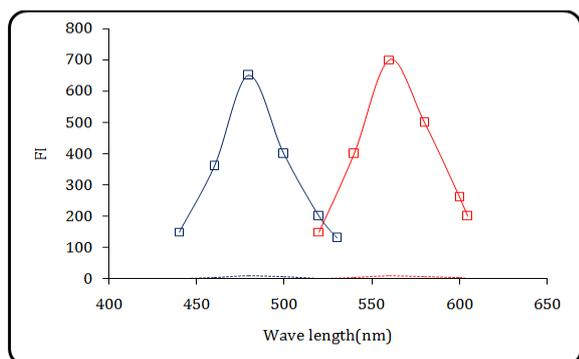
**Fig. 3: Fluorescence spectra of (a, b) reaction product of APT (6µg/ml) with (0.8% w/v) MAA, (a, b) blank of (0.8% w/v) MAA**
