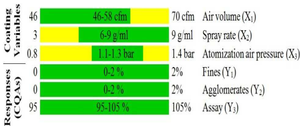
Fig. 6: The control strategy for pantoprazole enteric coating process
