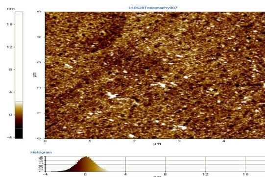
Fig. 5: AFM image of GCBNP 3 nanoparticles
