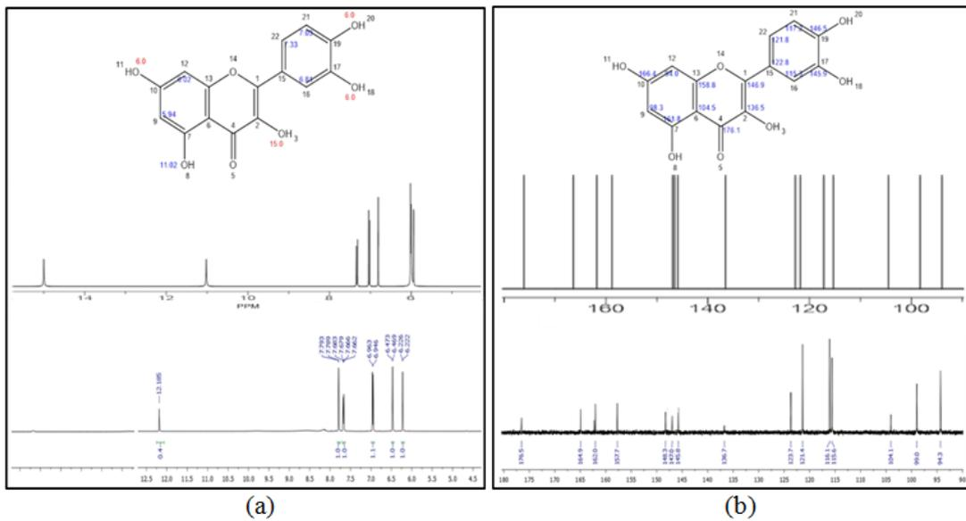
Fig. 6: <sup>1</sup>H-NMR (a) and <sup>13</sup>C-NMR (b) spectra of quercetin by computational prediction (upper) and laboratory experiment (lower)
