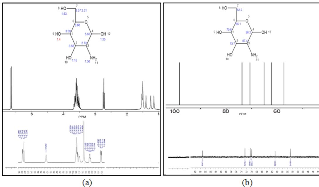
Fig. 7: <sup>1</sup>H-NMR (a) and <sup>13</sup>C-NMR (b) spectra of glucosamine by computational prediction (upper) and laboratory experiment (lower)
