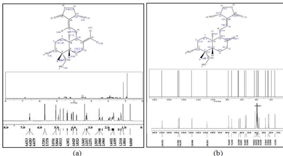
Fig. 8:  $^1\text{H-NMR}$  (a) and  $^{13}\text{C-NMR}$  (b) spectra of andrographolide by computational prediction (upper) and laboratory experiment (lower)
