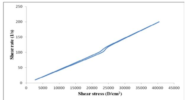
**Fig. 5: Rheogram for the micro emulsion using rotational viscometer**
