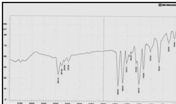
Fig.3: infrared spectrum of the compound 4-alkoxy banzaldehyd
