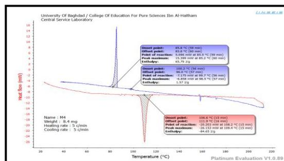
Form (4) curve differential scanning Calorimeter compound M4
