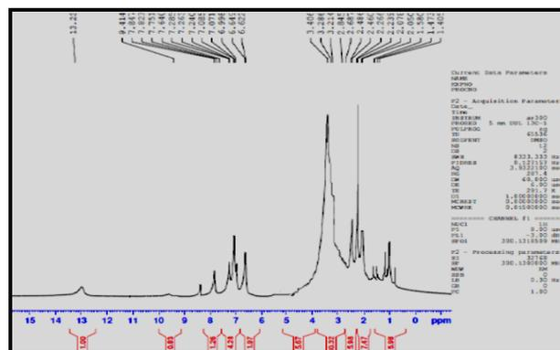
1. peaks at (0.90-1.80)ppm due to alkyl groups (CH<sub>3</sub>CH<sub>2</sub> CH<sub>2</sub> CH<sub>2</sub>)
