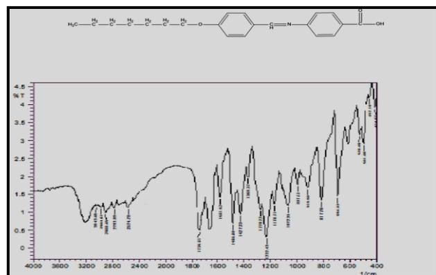
**Fig.5: infrared spectrum of the compound C7**
