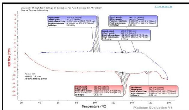
Form (3) curve differential scanning Calorimeter to compound C7
