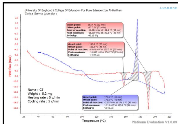
Form (1) curve differential scanning Calorimeter to compound C3
