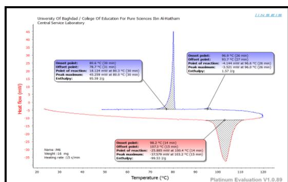
Form (5) curve differential scanning Calorimeter compound M6
