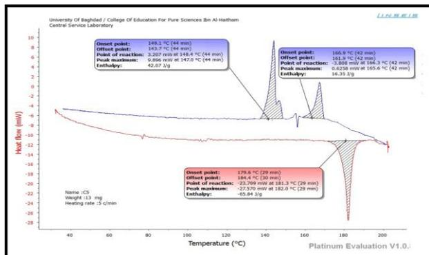
Form (2) curve differential scanning Calorimeter to compound C5
