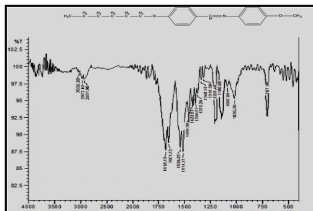
**Fig.7: infrared spectrum of the compound M6**
