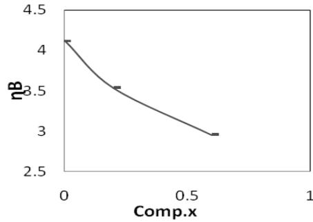
Fig. 3: Variation of magneton number ( $n_B$ ) versus comp.x
