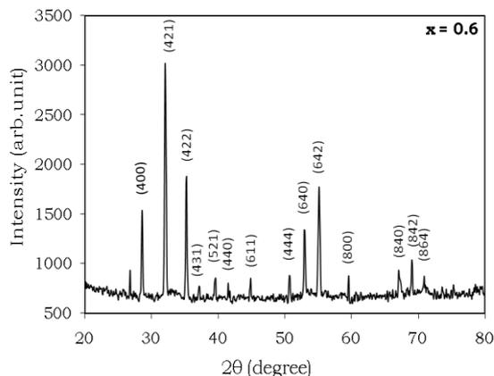
Fig. 1: Typical XRD patterns of  $Y_3In_xFe_{5-x}O_{12}$ . ( $x = 0.2$  and  $0.6$ )
